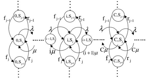
**Figure 2: State transitions for M/M/C queue with deteriorating service**
